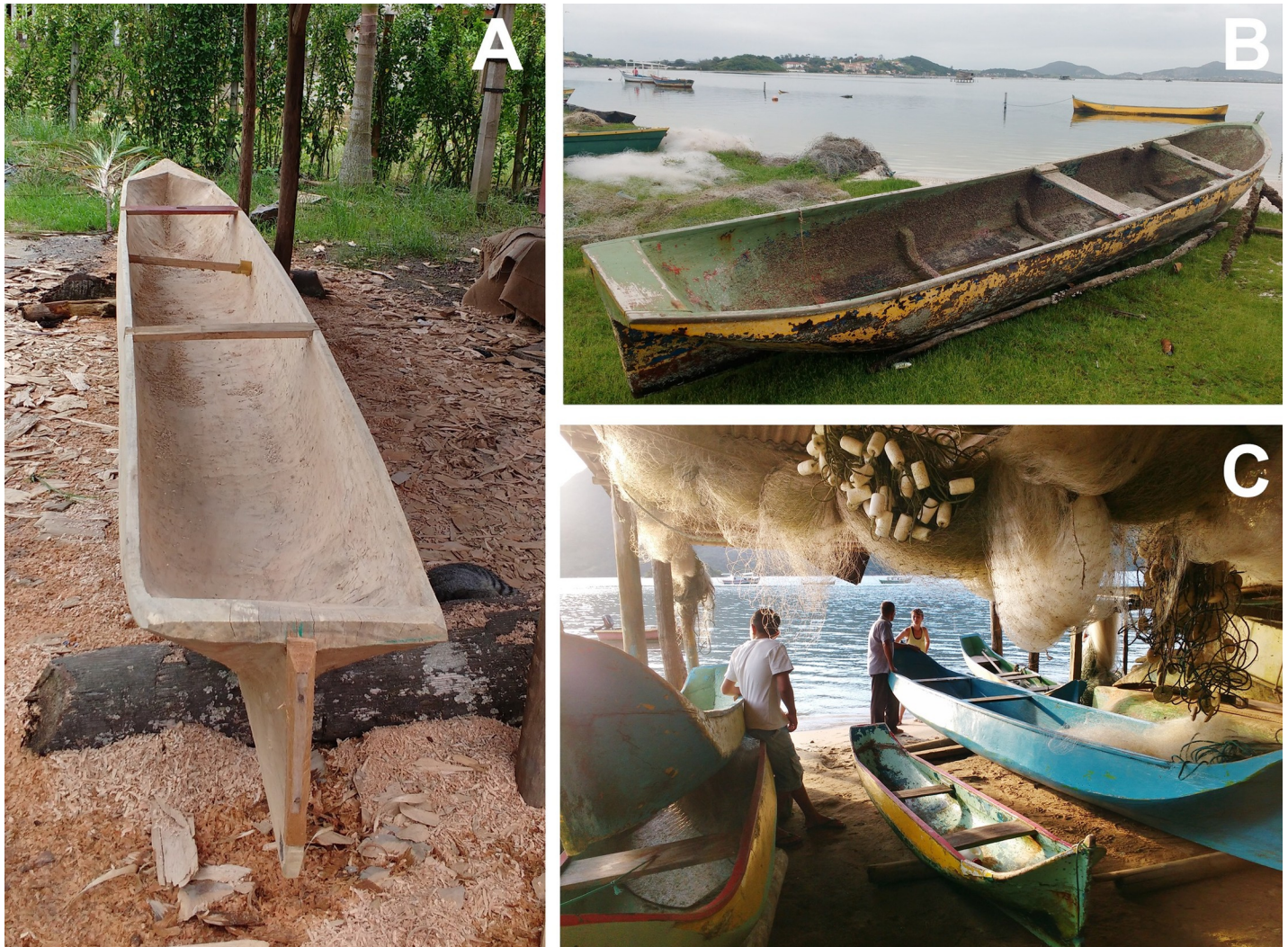
Fig 2. Examples of the canoes sampled. (A) Canoe under construction in Antonina (Paraná State, R3), made with Vochysia bifalcata , length 5.9m; (B) Canoe with about 70 years old in São Pedro da Aldeia (Rio de Janeiro State, R1), made with Clarisia racemosa , length 6.44; (C) Several canoes in Saco do Mamanguá (Rio de Janeiro State, R2): large blue canoe with 17 years made of Tachigali sp., 7.6m length; small yellow canoe with 16 years made of T. denudata , 3.13m length.
